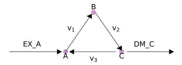
While this model contains a loop, a flux state exists which has no flux through reaction  $v_3$ , and is identified by loopless FBA.
